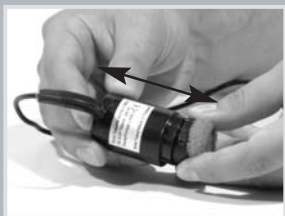
Remove pump base
