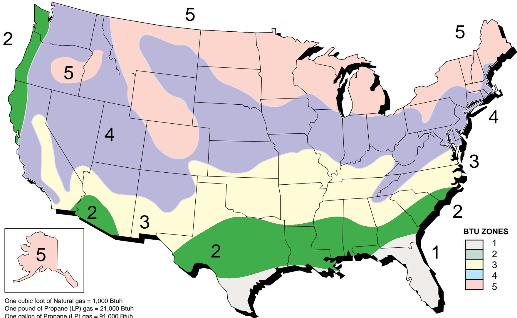
This chart is for rooms with average insulation and windows for your Btu zone. The sizing chart is based on a 72° temperature. To maintain higher room temperature, use the next higher Btu zone.
